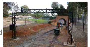
When a train arrives at the approach track section of the Main Line or Loop Line the signal controlling that movement will clear the signal provided the track is clear.
